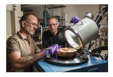
Sandia Labs' Mark Reece, left, and Don Susan examine a new shape memory alloy button they have removed from an arc-melter. | Credit: DOE
