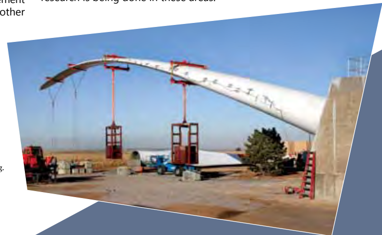
Deflection of a cantilevered 45-meter blade under distributed static load testing. Fundamentals of Materials for Energy and Environmental Sustainability (2012).
