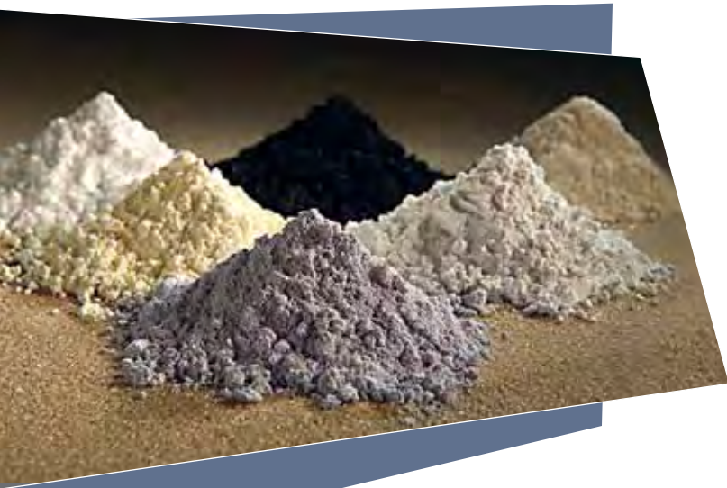
Rare-earth oxides, clockwise from top center: praseodymium, cerium, lanthanum, neodymium, samarium, and gadolinium. Wikimedia Commons .
