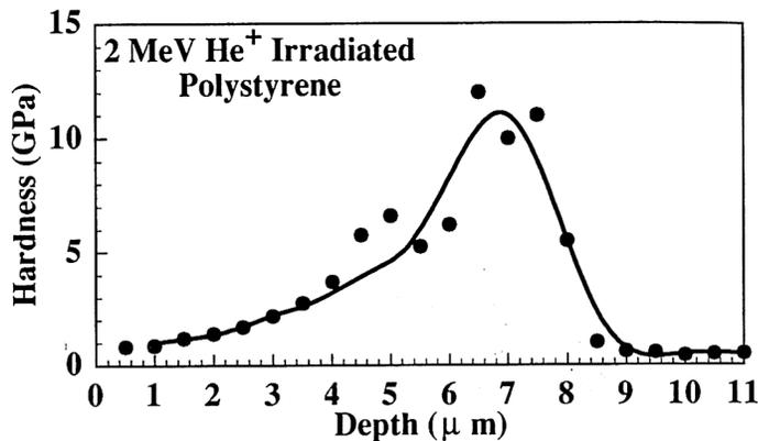
**Figure 1.** Nanoindentation hardness values as a function of irradiation depth (data points) taken across the cross-section showing a peak hardness of 12 GPa at a depth of approximately 6.5  $\mu\text{m}$ . (*Example E*)
