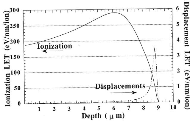
**Figure 2.** Ionization and displacement Linear Energy Transfer (LET) profiles for 2 MeV He<sup>+</sup> irradiation of polystyrene. The peak of the ionization profile corresponds to the peak hardness depth for the cross-sectional nanoindentation measurements in figure 2. (*Example E*)
