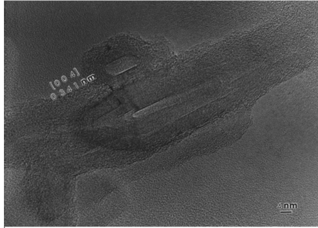
Figure 4 Electron micrograph showing the typical polyhedral forms encountered in WS 2 .
