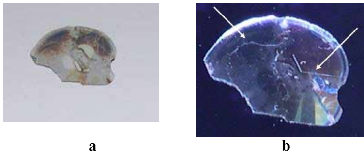
Fig. 2 Cracking in AlN samples: a) optical image and b) corresponding birefringence image. Cracks are marked by the white arrows.
